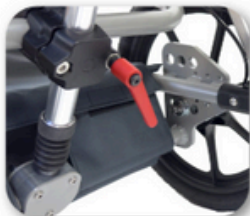
Seat angle adjustment and suspension
